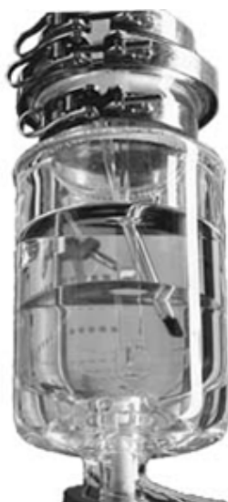
Figure 3 The BASIL™ process. After the reaction two clear liquid phases are obtained; the upper one is the pure product and the lower is the ionic liquid HMIMCl (© BASF Aktiengesellschaft 2002).
